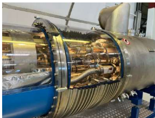
figure 13: LHC flexible joint manufactured by hydroforming
